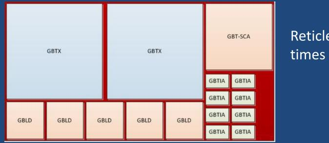
Reticle repeated 277 times on 8" wafer
