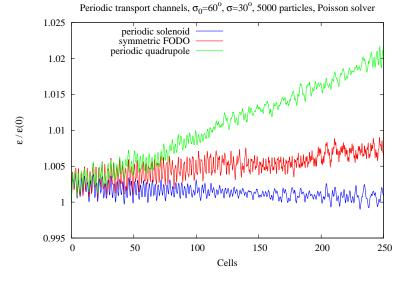
2*D* emittance growth factors versus number of cells for different focusing lattices,  $5 \cdot 10^3$  simulation particles, and 256 mesh points.
