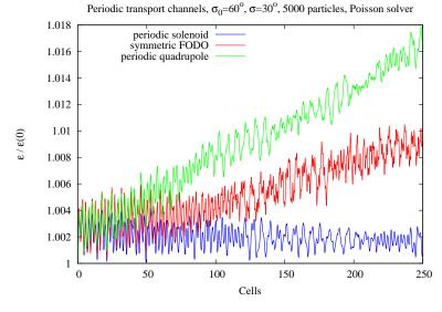
2*D* emittance growth factors versus number of cells for different focusing lattices,  $5 \cdot 10^3$  simulation particles, and 128 mesh points.
