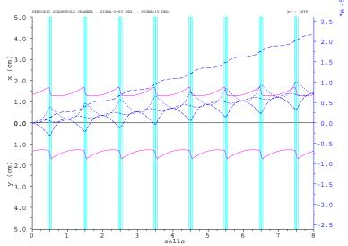
Beam envelopes (red lines) and emittance and momentum spread growth factors (dashed lines) in a FODO channel. The scale on the right hand side applies to the emittance growth functions.
