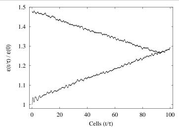
Emittance growth factors versus number of cells obtained by 3-D simulations of a periodic non-isotropic focusing system at  $\sigma_0 = 60^\circ$ ,  $\sigma = 15^\circ$  per cell, 2000 simulation particles. After 100 cells the time reversal occurs.
