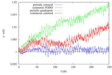
Normalized 2*D* emittance growth factors versus number of cells for different focusing lattices,  $5 \cdot 10^3$  simulation particles, and particle-particle interaction.
