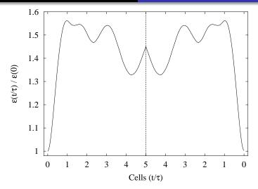
Emittance growth factors versus number of cells obtained for a non-stationary initial phase-space density at  $\sigma_0 = 60^\circ$ ,  $\sigma = 15^\circ$ , 2500 simulation particles.
