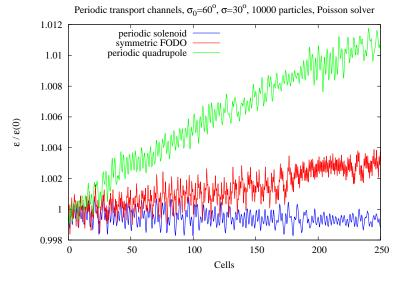
2D emittance growth factors versus number of cells for different focusing lattices, 10<sup>4</sup> simulation particles, and 256 mesh points.
