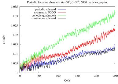
2D emittance growth factors versus number of cells for different focusing lattices,  $5 \cdot 10^3$  simulation particles, and particle-particle interaction.
