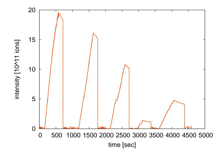
Reduced injection efficiency due to mis-steering
