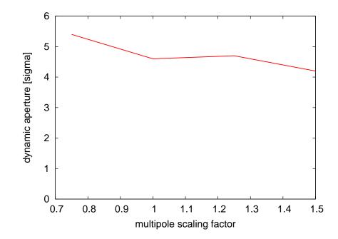
Minimum DA drops from  $4.6\sigma$  to  $4.2\sigma$  when all multipole errors are increased by 50 percent (Note that increasing  $b_2$  changes the machine sextupoles, which may explain the plateau) Beam-beam in the presence of space charge
