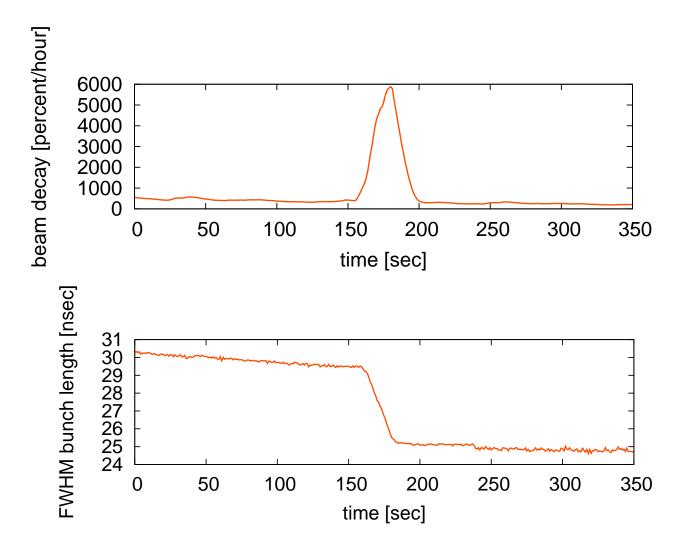
Beam decay immediately recovers when tunemeter is turned off Bunch length shrinks during kicking
