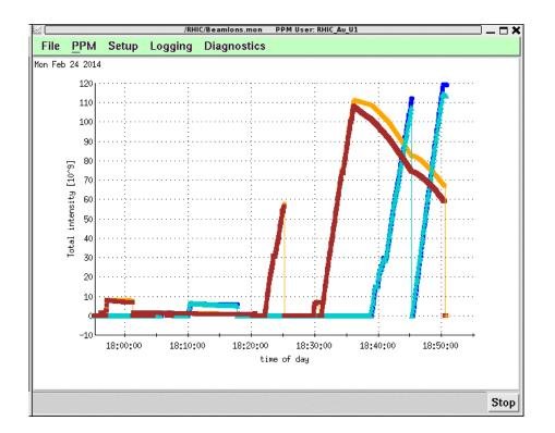
Yellow lifetime deteriorates as soon as Blue is injected
