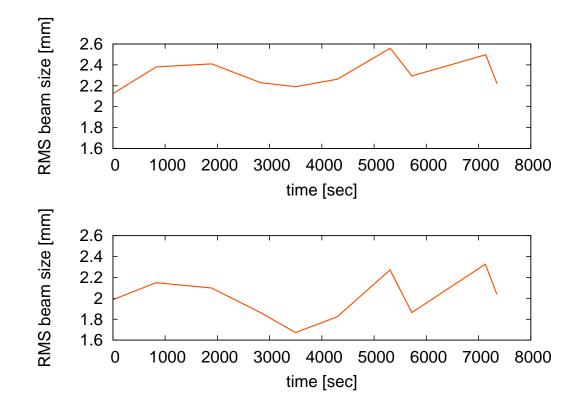
RMS beam size remains essentially unchanged regardless of mis-steering and tunemeter blow-up efforts - independent of intensity
