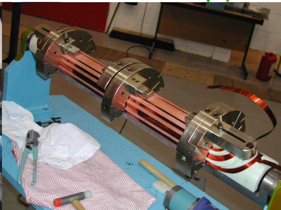
Dipole winding (MCBM)
