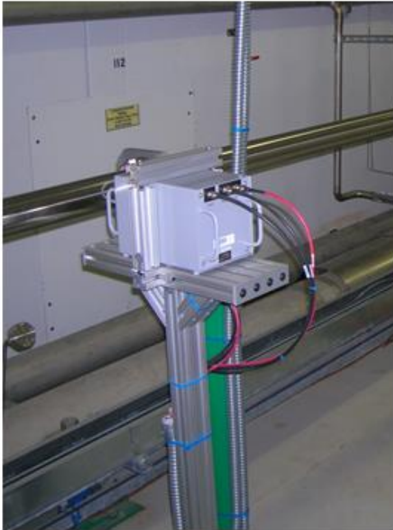
Figure 1: Neutron Detector is a 230x157x150mm box. PMT is inside x-ray shielding (lead) and is surrounded by polyethylene neutron moderator.
