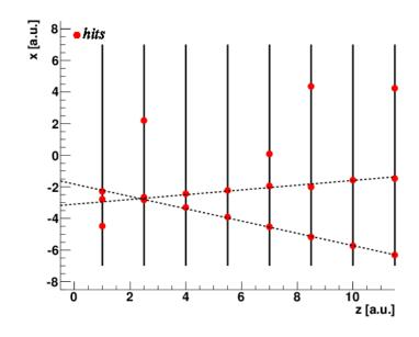
Discretize track parameter space in "cells". The center of each cell (or *d*-dim hyper-cube, in the case of a track with *d* parameters) identifies a track in the real space that intersects detector layers in "receptors".
