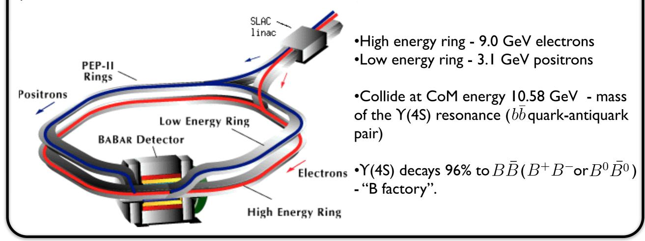
•BABAR collected data from 1999 to 2008 •Produced 471 million  $B\bar{B}$  pairs •429 fb<sup>-1</sup> integrated luminosity at Y(4S) resonance
