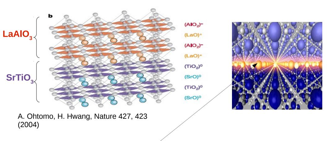
Conducting Interface OR Two-dimensional electron gas(2DEG)
