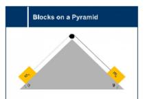
Exploration of free body diagrams, two body acceleration, and newton's laws through the system of two blocks resting on a pyramid and attached by a pulley.
