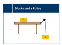
Exploration of free body diagrams, two body acceleration, and Newton's law through the system of two blocks attached through a pulley and one of them resting on a table.
