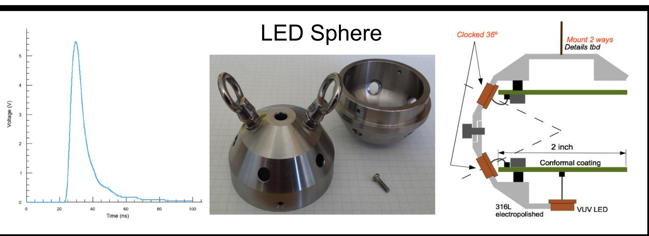
Figure 6 : 11 244nm LEDs are mounted in a dodecahedral pattern on a stainless steel source. The 12 th vertex is saved for the attachment point. The two eyelets on the sphere are attached to secondary bobbins to prevent the source from rotating. The LED driver is based on the Kapustinsky pulser and can produce 10ns wide pulses (FWHM).
