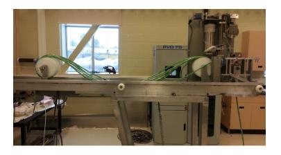
The Umbilical Retrieval Mechanism (URM) allows us to deploy the calibration sources to specific locations in the detector. Two original SNO URMs will be used in the water-fill phase.
