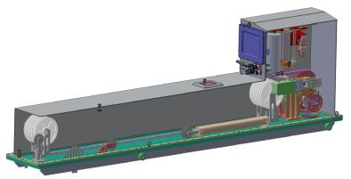
SNOLAB co-op students have been working on modifying the drive pulley system to increase the friction and tension needed to deploy a source precisely.
