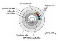
The umbilical contains a co-axial cable for a PMT and wires for positioning LEDs, which surround a central tube for the deployment of gaseous sources and contains quartz fibres for the Cherenkov source.
