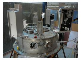
The Universal Interface (UI) connects the URM and the detector. It contains many sensors providing information about liquid levels and nitrogen cover gas quality, motor boxes for the side ropes that let us deploy sources off-centre, and glove ports for attaching sources. This effort is from TRIUMF.
