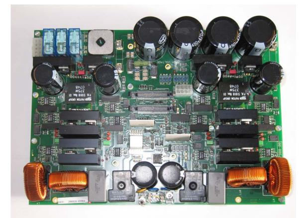
Redundant power part (over dimensioning hot spare)
