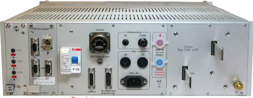
PC104 CAN bus to Ethernet controller Regulator Ethernet Connection
