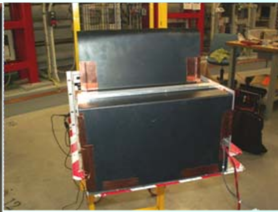
Temporary EMI Shield on the "Common Control Crate"
