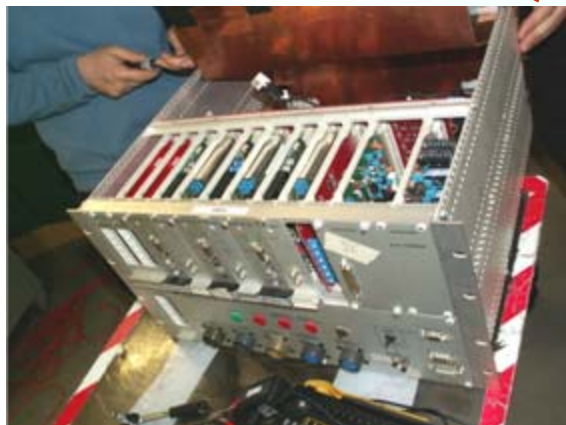
Temporary EMI Shield on the "Common Control Crate"
