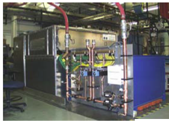
High Voltage Converter Modulator 140 kV, 70A, 1.6ms, 60 Hz Equipment Control Rack
