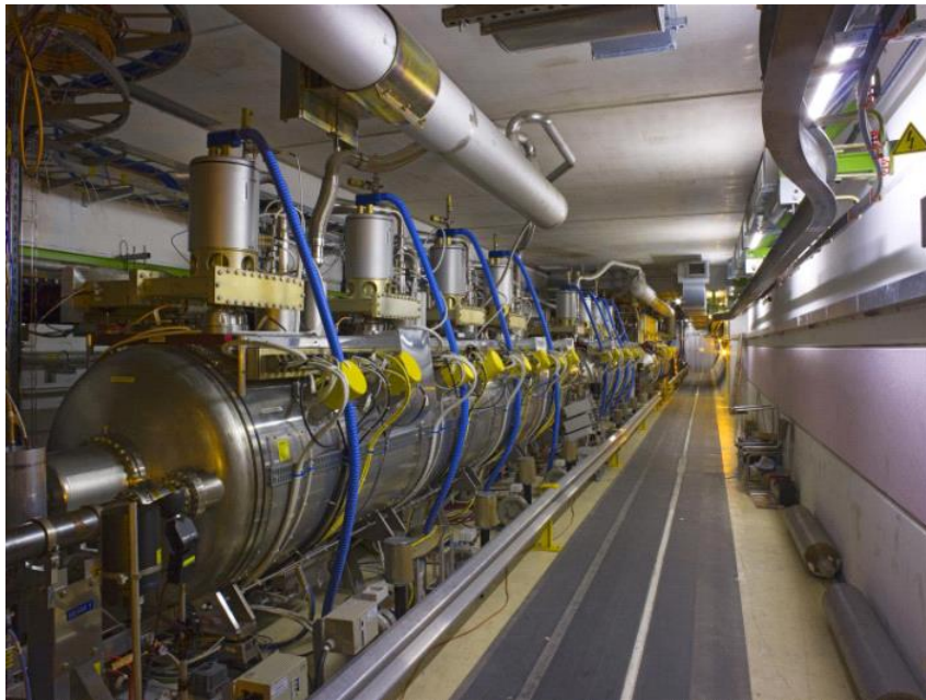
LHC 400MHz SC cavities
