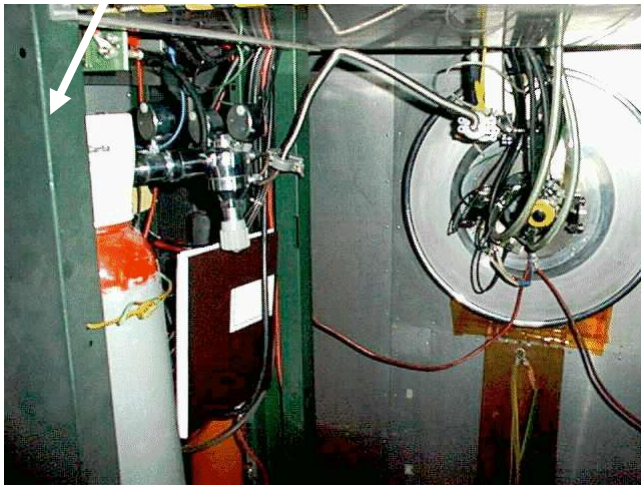
Hydrogen supply (one lasts for 6 months)
