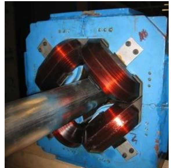
Measurement of quadrupole magnet
