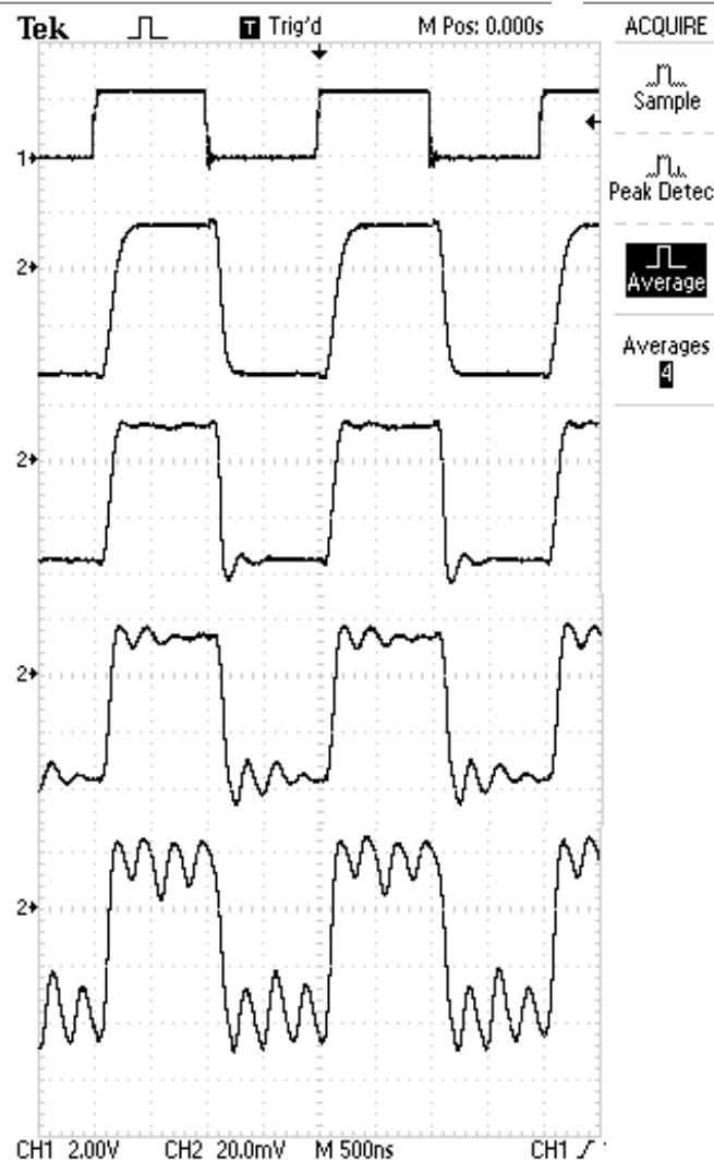
Mismatch ~13% reflected power at 100 deg towards load.
