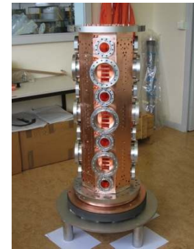
Design exists for ESS RFQ similar to 5 m long IPHI RFQ at Saclay. Energy 75 keV->3.6 MeV.
