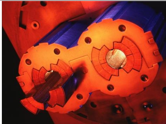
The LHC dipole; ultimate field >8T.
