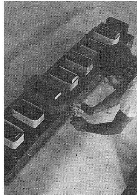
Figure 5 - Wiggler magnet for SPEAR (lower half) with seven full poles and two end half poles. Each pole is powered by a coil, only one of which is shown. (Photo by J. Faust, SLAC)
