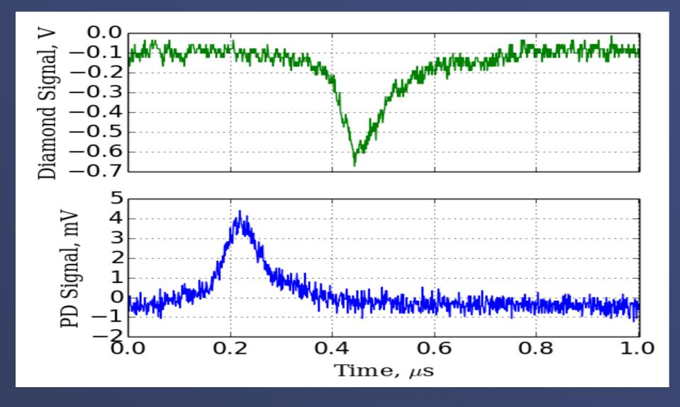
Automated vertical scans of the horizontal laserwire were performed for different diamond detector positions. At each step, diamond detector data were acquired in 30,  $1\mu$ s segments, for one accelerator macro-pulse. The laserwire position was then moved ready to acquire a subsequent accelerator pulse.
