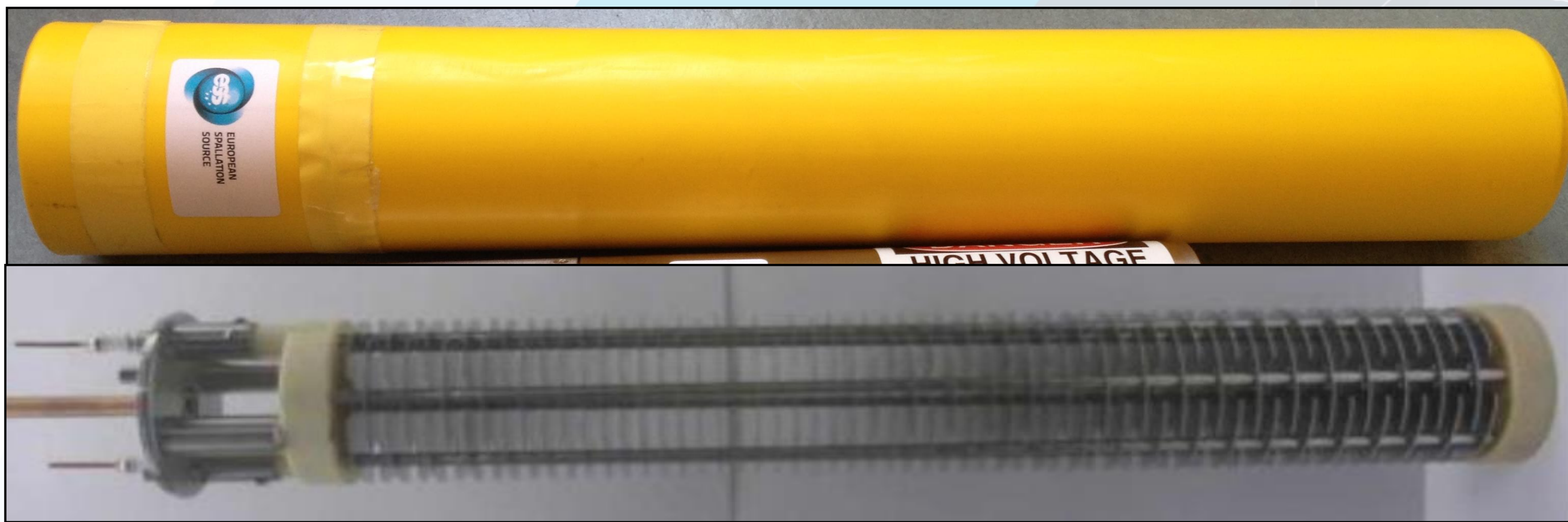
Figure 2: ESS Ionization Chamber with and without metal casing
