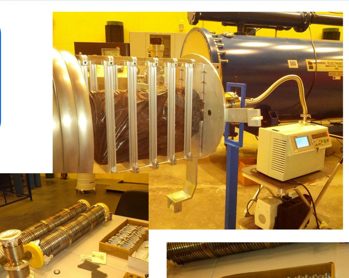
The leak was detected in second tube of low energy column.
