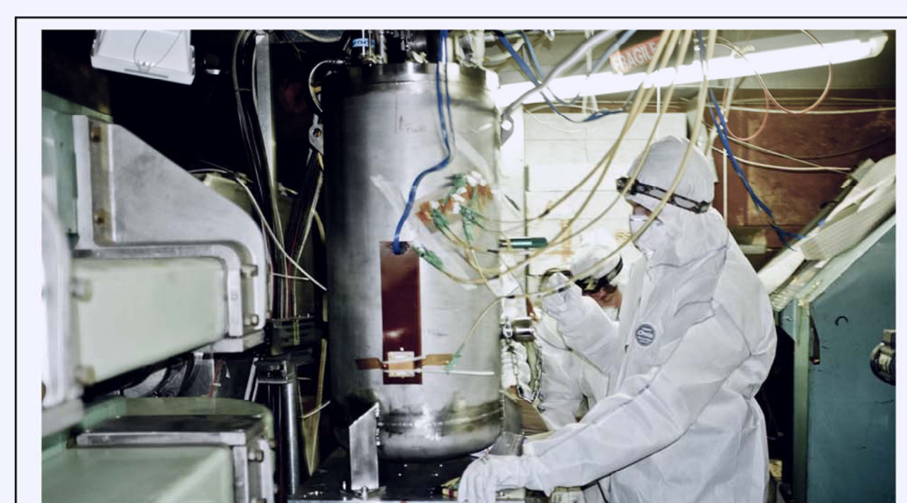
Figure 6: Preparation of the cryogenic irradiation test in T7 irradiation zone at CERN.
