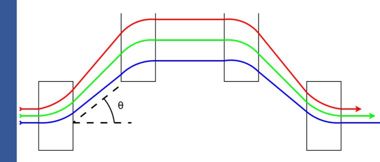
4 dipoles arranged in a chicane. Electrons with higher energy travel through longer paths than electrons with lower energy, resulting in a negative momentum compaction factor.
