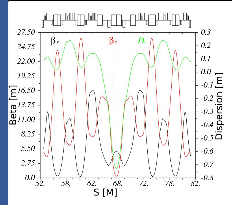
A chicane placed in one long straight section zero the  $\alpha$ :
