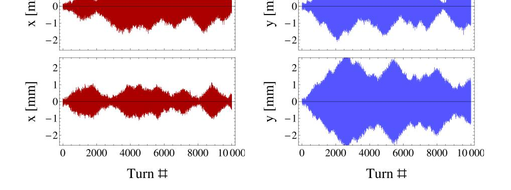
Simple tracking simulation including measured quad ripple, showing small and irregular beam response.
