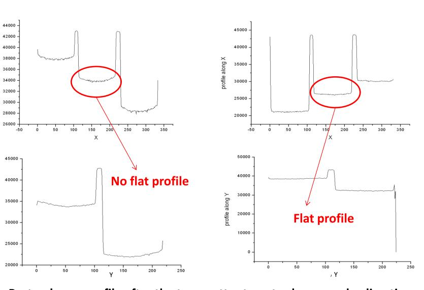
Proton beam profile after the two scatter targets along x and y directions
