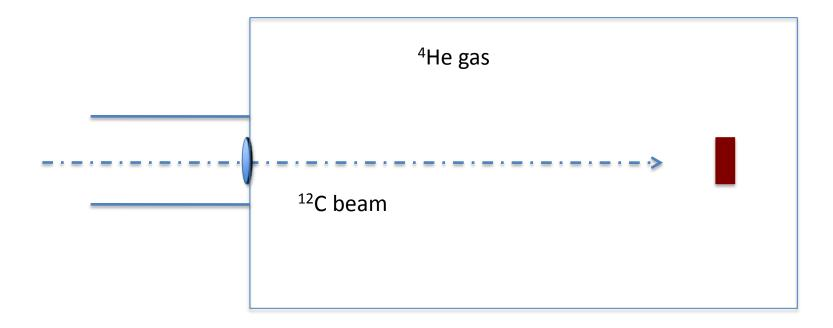
Sketch of the set-up. Detector at  $0^{0}$  with respect to the entrance window.
