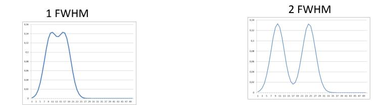
To have a satisfactory mass or charge identification two peaks differing by ONE mass or charge unit have to be separated by at least 2 FWHM. In other words:
