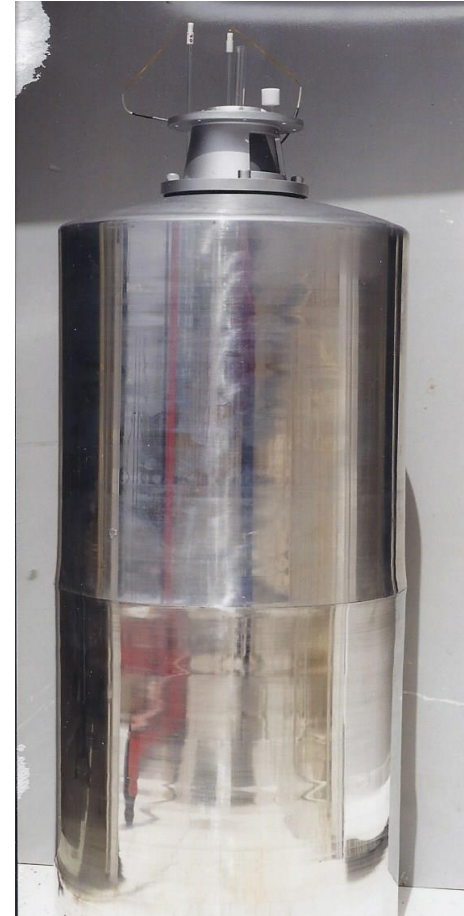
50 lt liquid Helium cryostat for materials testing (right)
