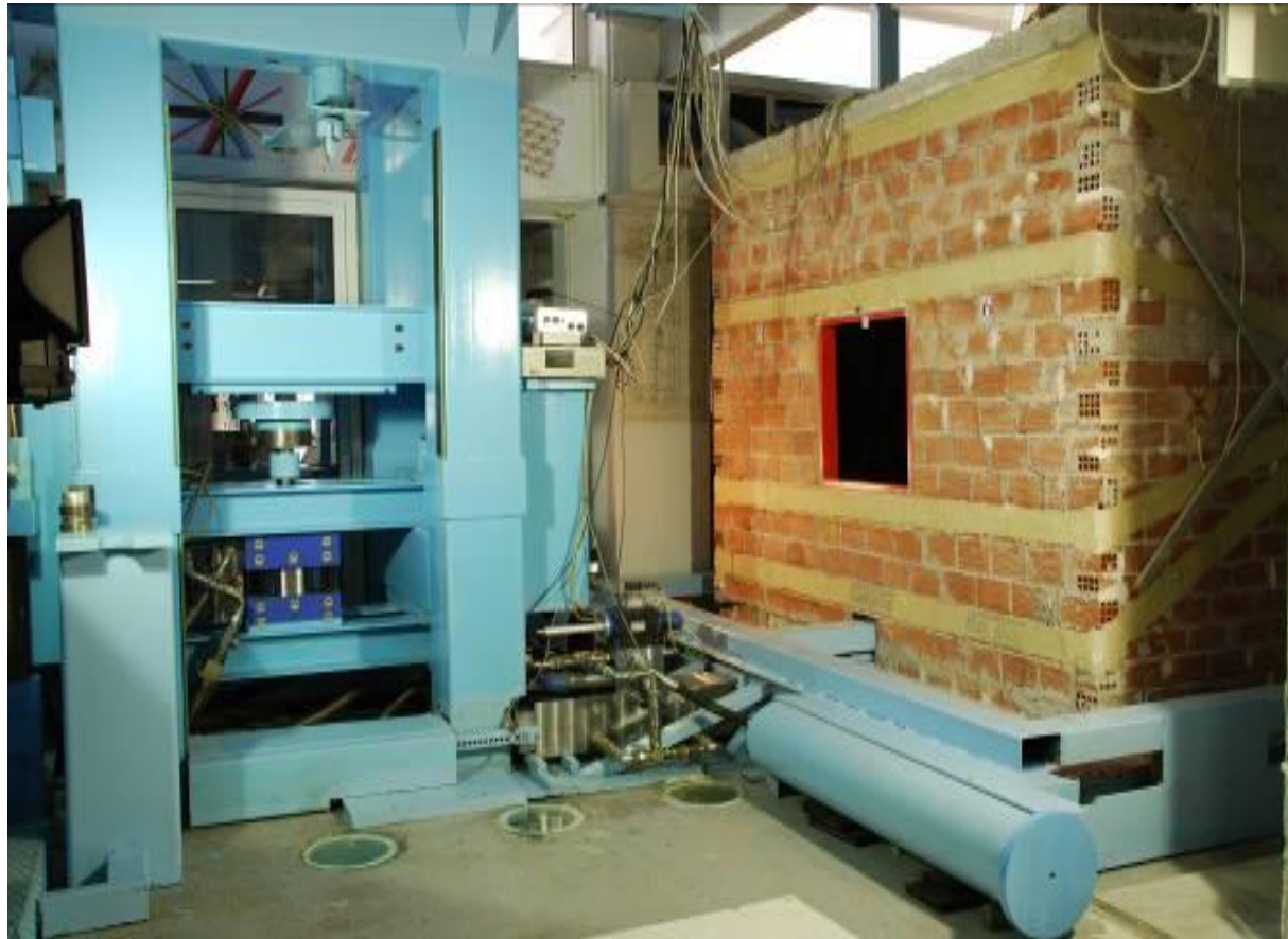
The actuation system of the IMMIG shaking table
