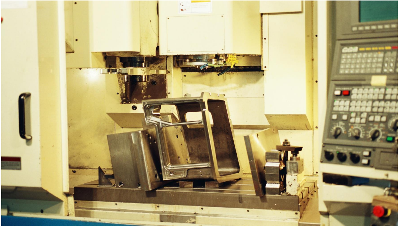
Machining one of the 320 optical systems housings for Leopard II MBT on the OKUMA MX45 VAE machining centre (2007)
