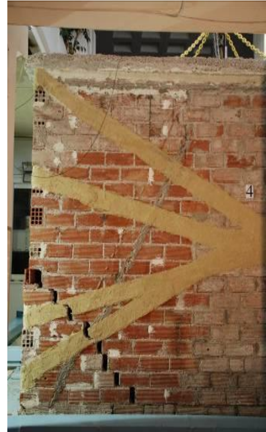
Damage inflicted on the masonry specimen tested at IMMG (unreinforced – left, repaired-reinforced – right)
