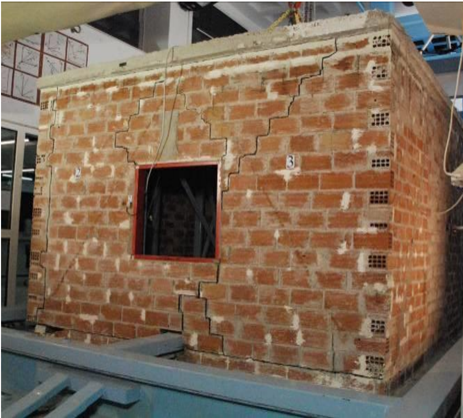
Damage inflicted on the masonry specimen tested at IMMG (unreinforced – left, repaired-reinforced – right)
