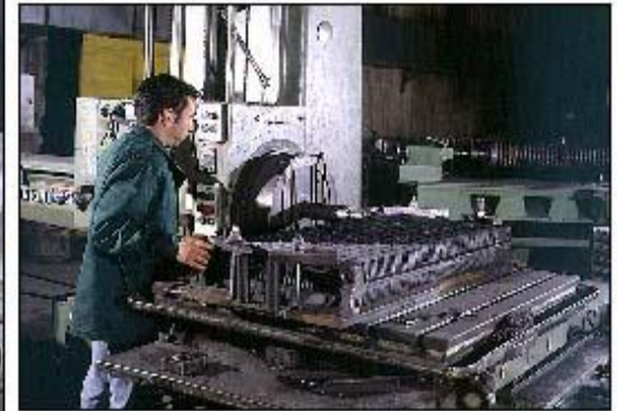
BORING – SHAFT \Phi 100
