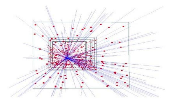
153 high energy particle tracks flying through a telescope of half a million pixels in the WA97 experiment back in 1995
