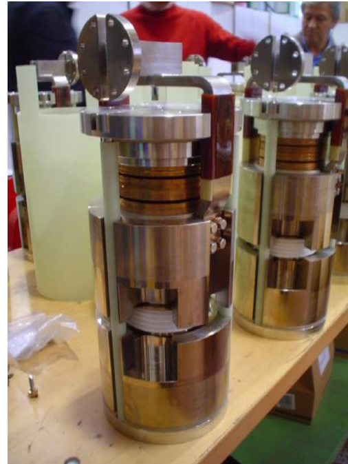
High current, radiation tolerant cold by-pass diodes for LHC main magnets.
