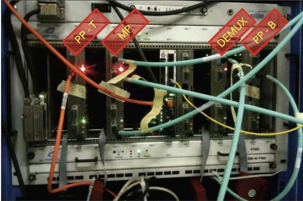
**Figure 4: Layer1 and Layer2 emulator inside a same MicroTCA crate with several MP7 cards**
