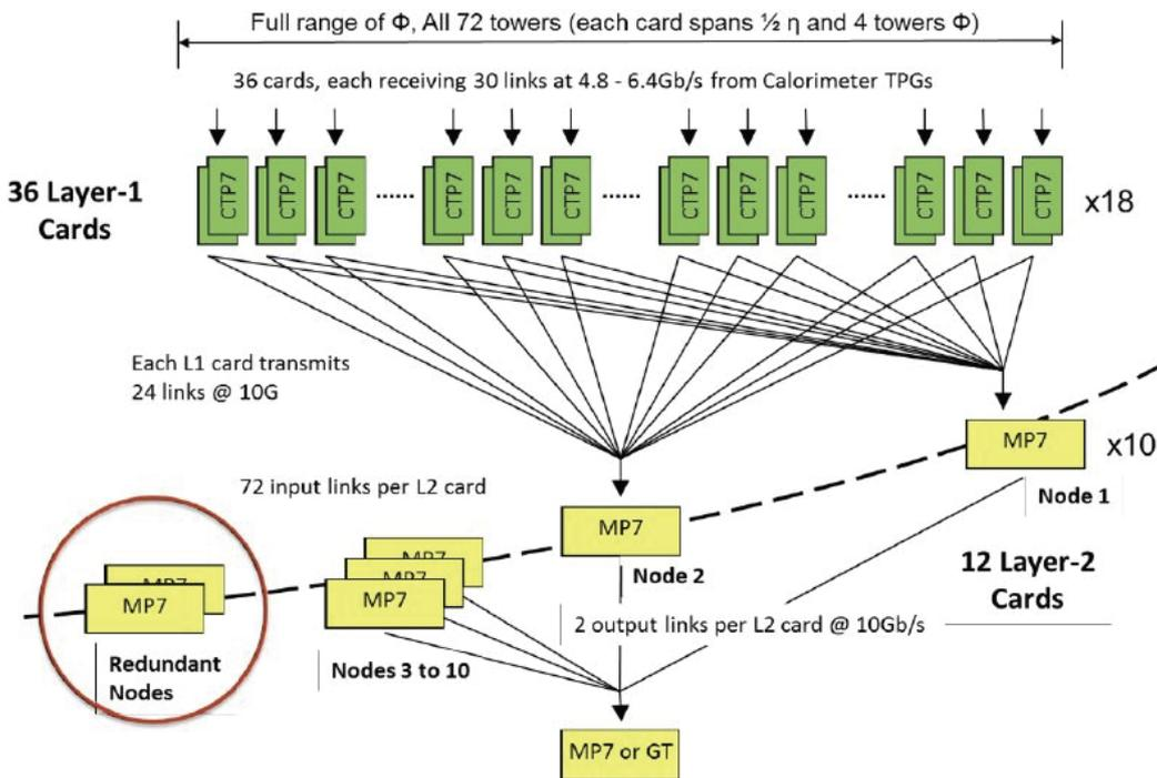
**Figure 1: TMT architecture for Trigger upgrade. Two output links from each CPT7 are connected to each MP7 (24 output of CPT7 to cover 12 MP7). On the MP7 side 72, serial links are used to connect to 36 CPT7 boards from Layer-1.**
