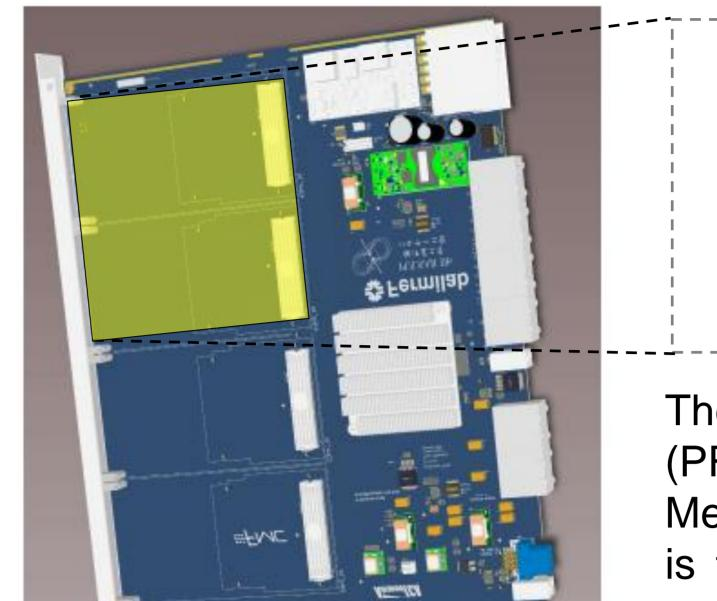
The Pattern Recognition Mezzanine (PRM), based on the Associative Memory and the FPGA technologies, is the mezzanine card to be hosted on Pulsar II mainboard to process the data.
