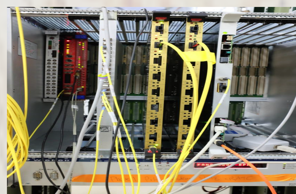
Upgraded Pixel FED w/two daughterboards and controllers.
