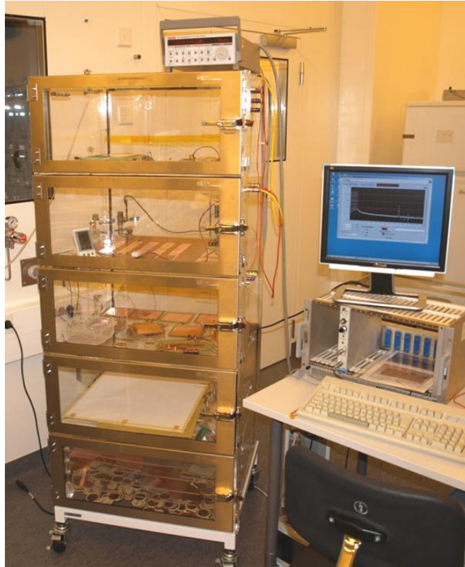
Figure 4.21: Leakage current measurement setup.
