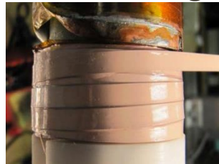
Polyester heat shrink tubing from Advanced Polymers, Inc., used for Y10-04 test coil at NHMFL
