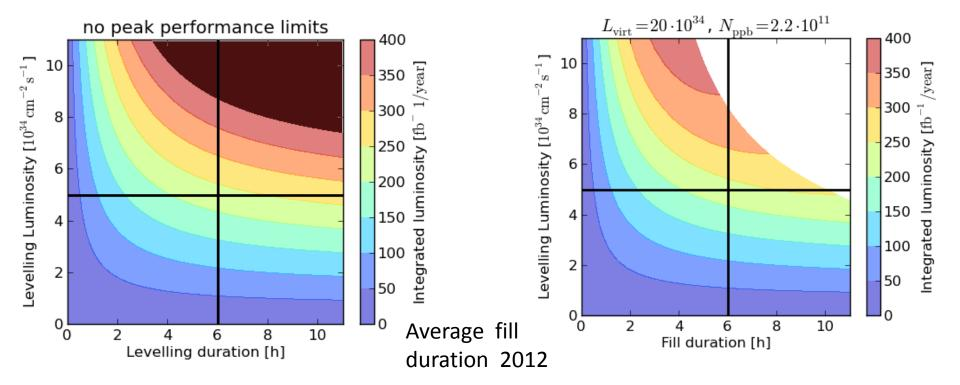
Adding a simple model of peak machine luminosity and burn-off decay (F. Zimmerman).
