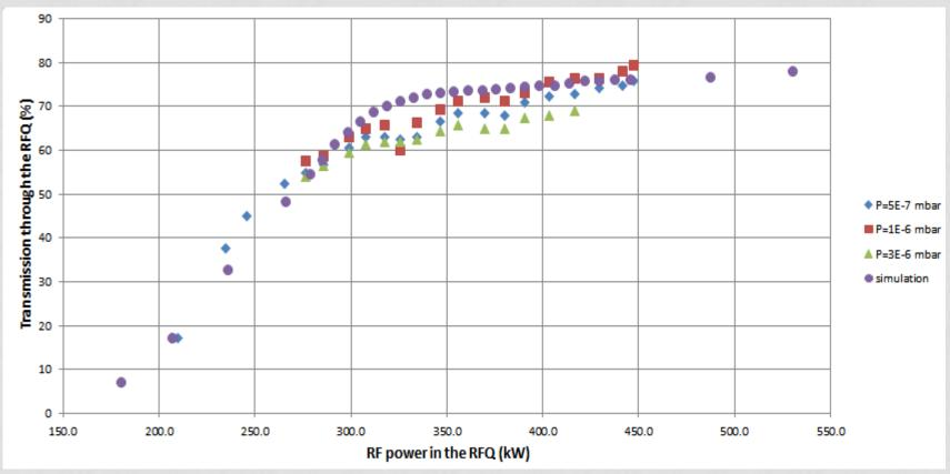
RFQ Transmission vs. RF power for different pressure in the LEBT (neutralisation)
