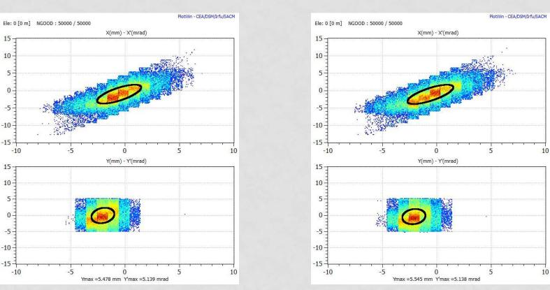
Emittance measured with chopper off (left) and with chopper on (right) downstream the inline dump
