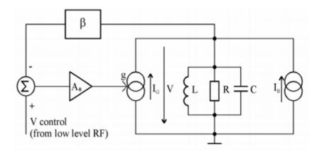
R= final resistance of the amplifier and cavity losses  $I_G$  = provided by the power RF amplifier  $I_B$  = current due to the beam producing a voltage in the cavity called **Beam loading voltage**  $V_B$ V = total voltage in the cavity ( $V_{GAP}$ )
