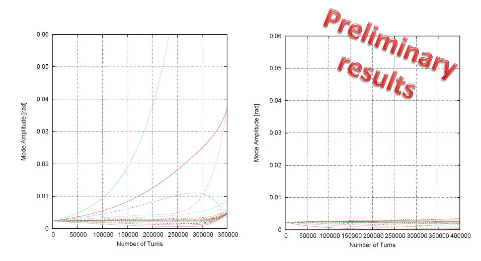
Simulations performed with 21 bunches IN h=21 with an intensity of  $2.7 \cdot 10^{11}$  ppb at extraction.
