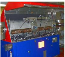
The **10 MHz cavity** with a power up to 20 kV, it is tuneable from 2.8 MHz to 10.1 MHz, h = [6...21].
