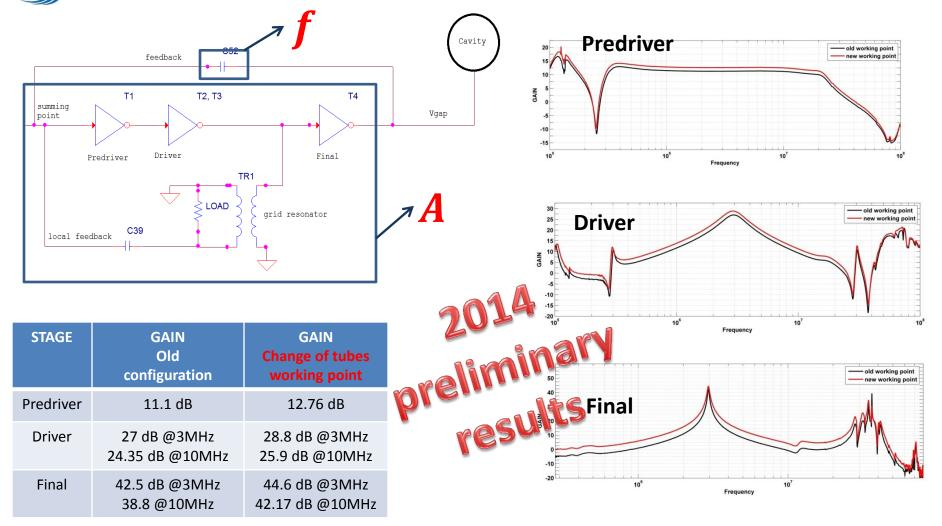
**TO DO NEXT** -> verify that with the new working points the amplificator (in the limit of stability and respecting the phase and gain margin) give to the cavity 10 kV per gap.
