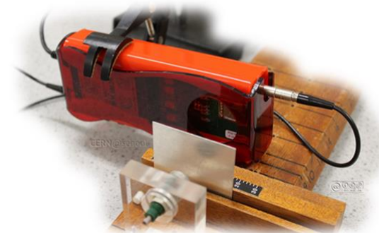
Experimental arrangement for investigating the attenuation of beta radiation with a radioactive source.
