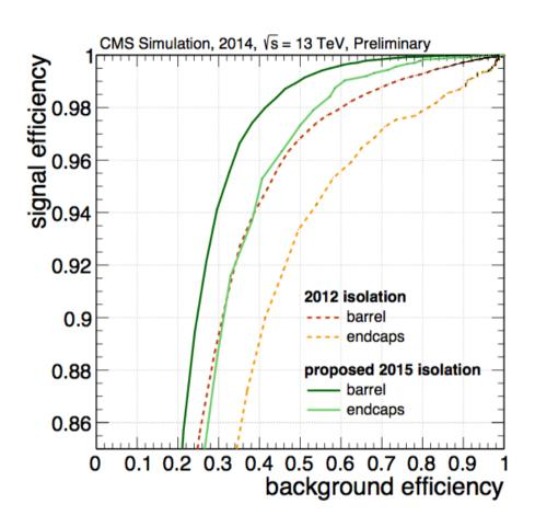
• improved **electron isolation** based on particle flow reconstruction
