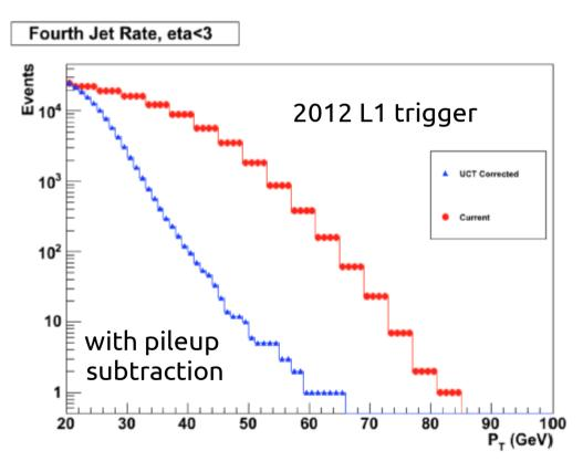
effect of pile-up subtraction on energy sums and multi-jet trigger
