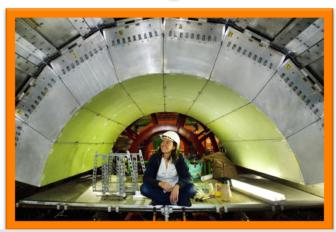
Homogeneous, hermetic, high granularity PbWO<sub>4</sub>crystal calorimeter
