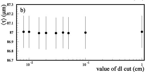
MC corrected measured values of the  $\tau$  lifetime as function of the value of the cut on dl
