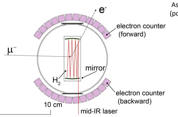
Detector Solid angle ~28% each Asymmetry factor (polarization sensitivity )~0.23
