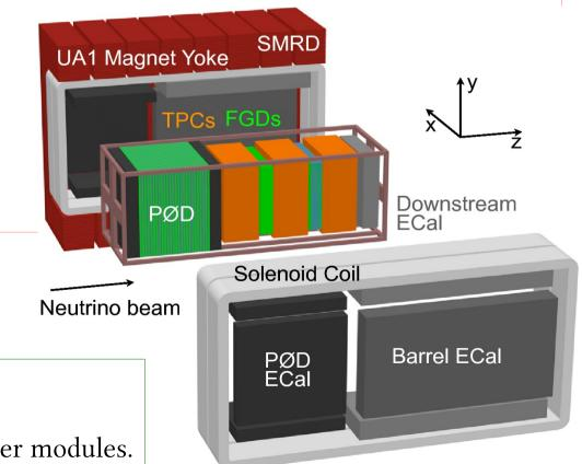
\*2FGDs: First FGD is fully scintillator (CH). Second FGD is divided into scintillator and water modules.
