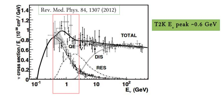
Data collected in the near detector of the T2K experiment provide a coverage of the critical low to intermediate energy region
