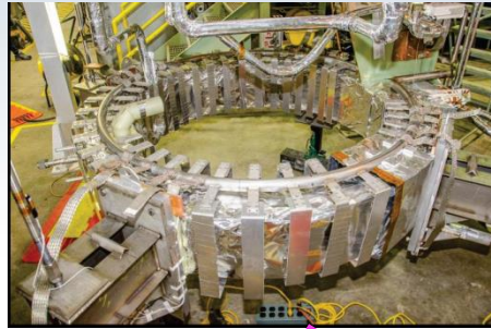
CC cold mass under test at Fermilab
