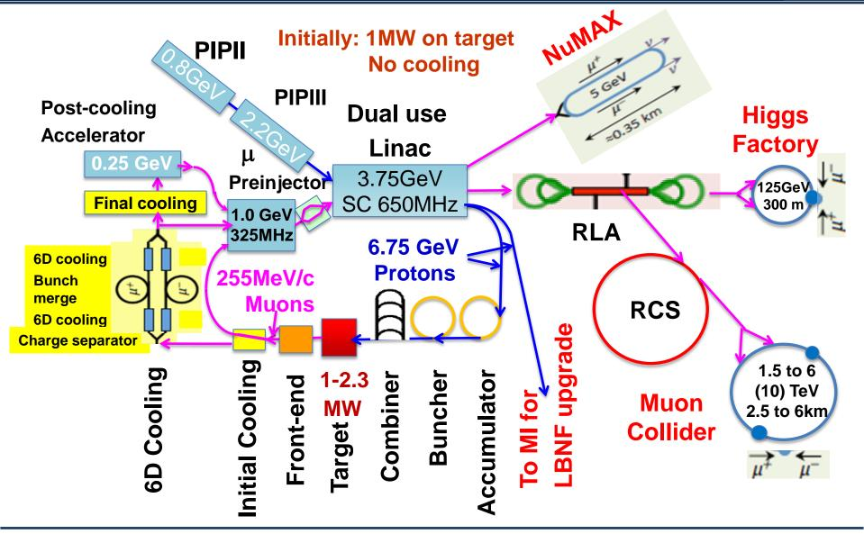
**A Potential Muon Accelerator** Complex at Fermilab: vSTORM -> NuMAX → Higgs Factory 0.8 GeV Proton Linac (PIPII)
